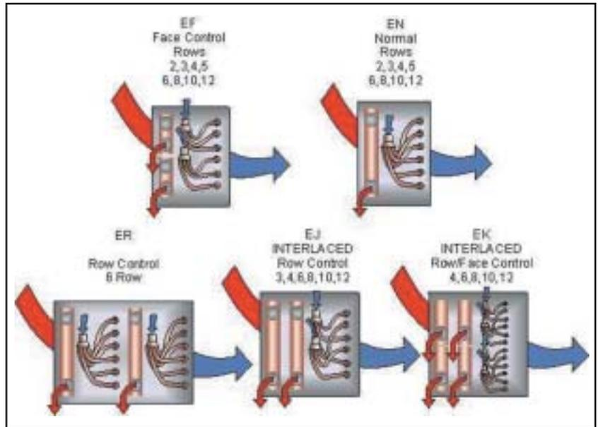
THERE ARE ALSO DIFFERENT TYPES OF EVAPORATORS THAT HAVE VARYING TUBE PATTERNS AND FIN SURFACES. THE TYPE OF EVAPORATOR CHOSEN CAN DETERMINE HOW MUCH MOISTURE IT CAN PULL FROM THE AIR. SOME OF THE DIFFERENT TYPES OF FIN SURFACES AVAILABLE ARE A FLAT FIN, A CORRUGATED FIN, AND A SINE-WAVE FIN.
