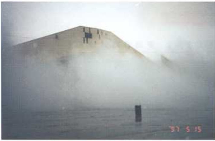
Air cooled to -65°F instantly turns to fog as it exits the chamber into the humid Florida air.
